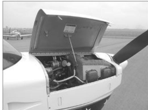
Engine access is via a split cowling.
